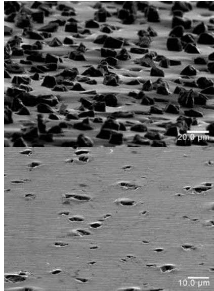
Fig. 2: Contact surface of friction joint with EKagrip® friction enhancing shim after assembly and disassembly
