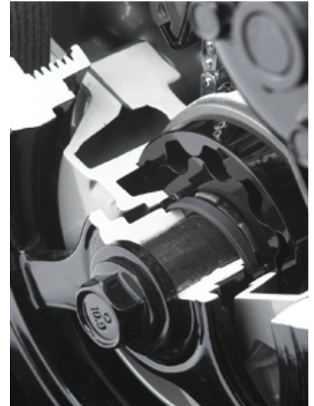
EKagrip® friction shim in the GM L5 crankshaft application
