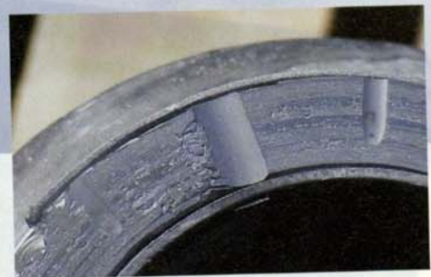
Fig. 3. Overloaded axial bearing of standard SSiC.
