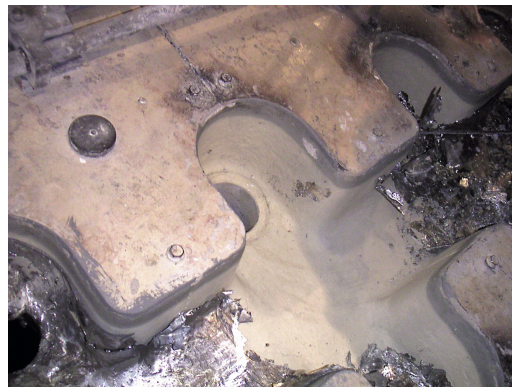
Casting table for aluminum billet production coated with EKamold Cast-C after use
