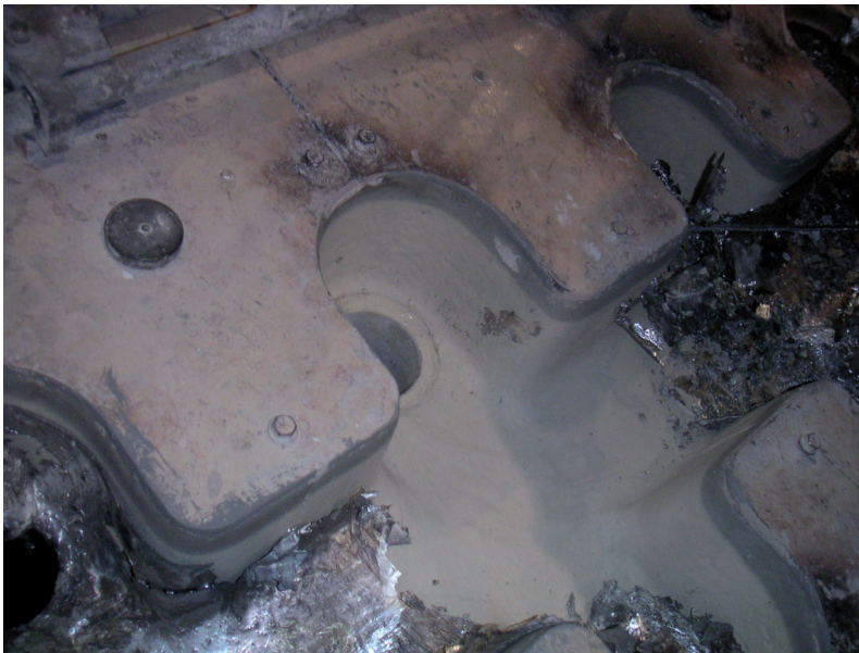
Fig. 2: Casting table for aluminum billet production coated with EKamold® Cast-C after use
