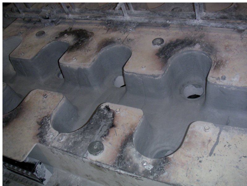
Fig. 1: Casting table for aluminum billet production coated with EKamold® Cast-C prior to use
