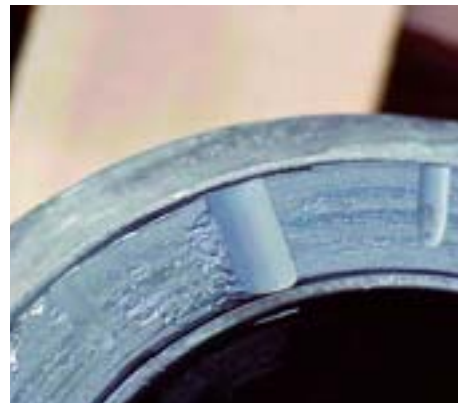
Overloaded thrust bearing made of standard SSiC
