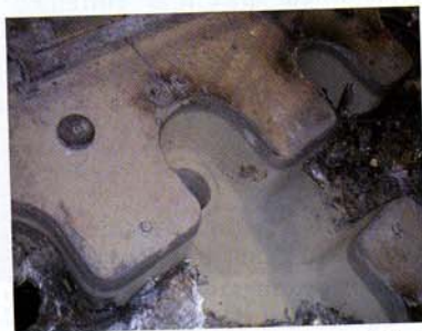
Casting table for aluminum billet production coated with EKamold® Cast-C after use
