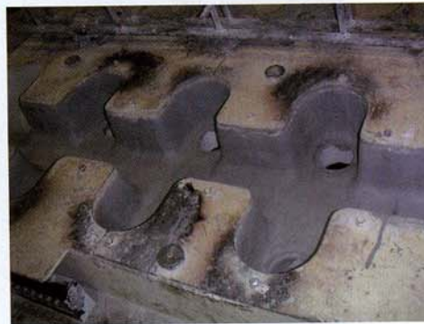
Casting table for aluminum billet production coated with EKamold® Cast-C prior to use
