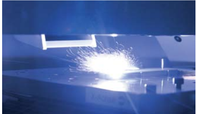
3D-microstructuring by an ND:YAG laser.
