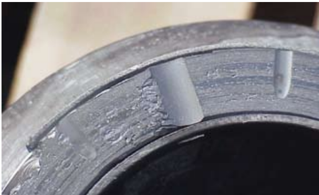
Overloaded thrust bearing of standard SSiC.
