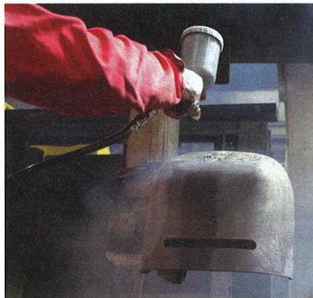
Quick and easy recoating of a hot casting ladle with ESK's EKamold® Cast-M suspension for metal substrates
