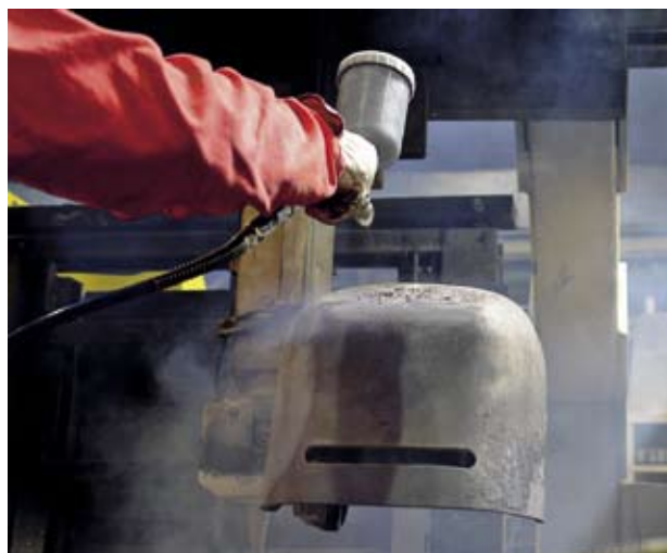
Quick and easy recoating of a hot casting ladle with ESK's EKamold Cast-M suspension for metal substrates
